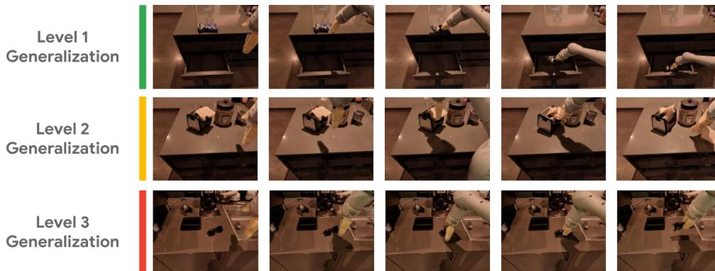
Figure 11: “Realistic instructions” evaluations propose realistic scenarios multiple distribution shifts that incrementally increase in difficulty.  $L1$  generalization introduces a new real office kitchen with new lighting conditions.  $L2$  generalization additionally adds unseen distractor objects. Finally,  $L3$  generalization includes new objects or objects in new locations, such as next to a sink.
