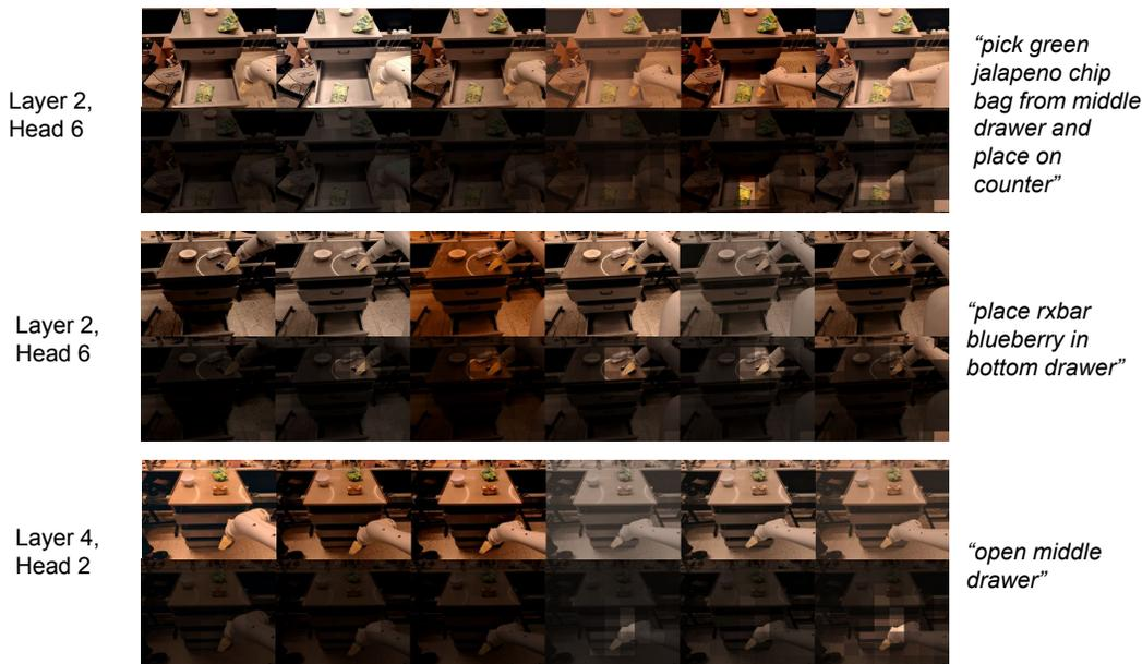
Figure 13: In this figure we show the attention map of the RT-1 policy. Different layers and heads generally focus on different part of the image. Most commonly, they focus on the parts of the scene with the richest interaction affordances, such as graspable objects. For example, Layer 2 Head 6 focuses on the jalapeno chips and pepsa can in grasping tasks; and Layer 4 Head 2 focuses on the drawer in drawer opening tasks.
